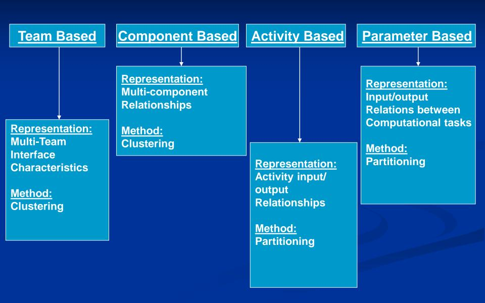
Static DSM represents system elements existing simultaneously, such as components of product architecture or groups in an organization.
